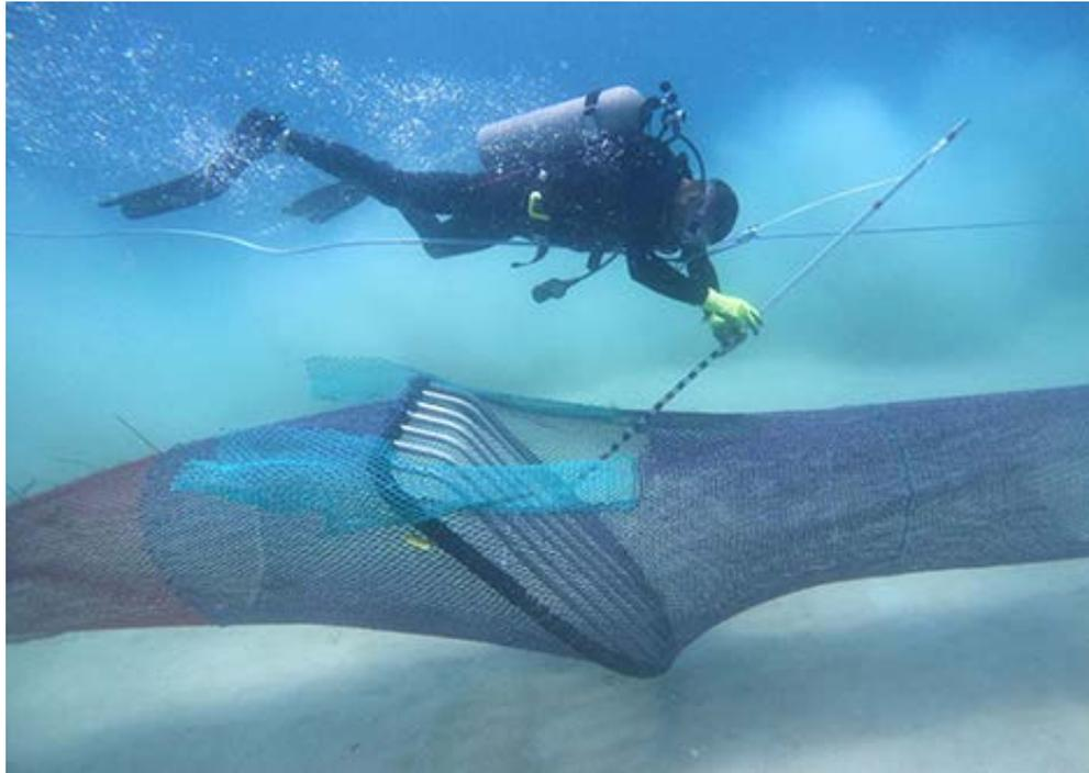
Three candidate devices tested to reduce fish bycatch
